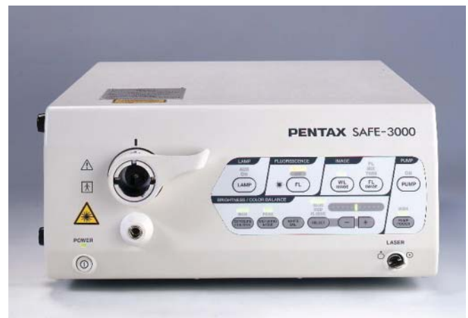
FIGURE 2. Pentax SAFE 3000® (Pentax Corp., Tokyo, Japan) autofluorescence bronchoscopy system.
